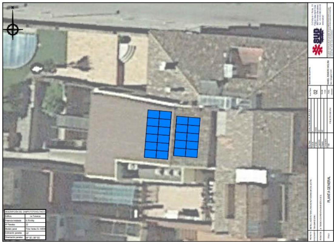
Figure 2. Collective PV installation on the bishopric roof
